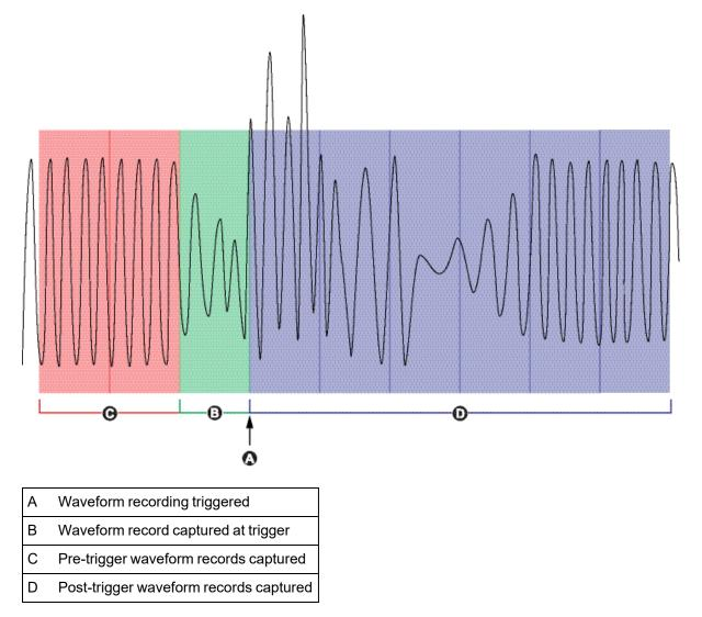
The waveform log set for each triggered recording is equal to the sum of *Pre-trigger Records* + *Post-trigger Records* + 1 (where 1 is the actual record when the Waveform Recorder module's *Record* input was triggered).
