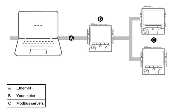
To use the Modbus client-server architecture, add the Modbus server devices using ION Setup.
