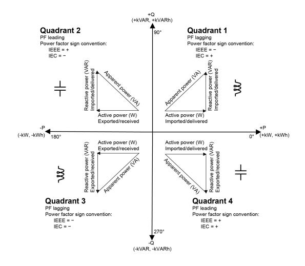
The units for power are watts (W or kW) for real power P, vars (VAR or kVAR) for reactive power Q, and volt-amps (VA or kVA) for apparent power S.
