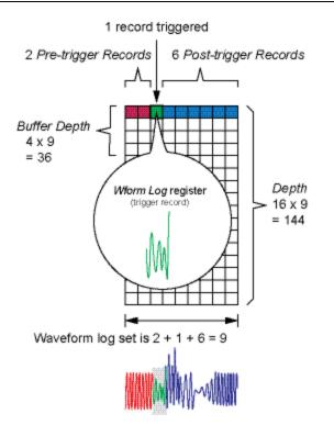
The waveform log set for the extended waveform capture = [pre-trigger records] + [actual trigger record] + [post-trigger records]. The total waveform records captured in this example is 2 + 1 + 6 = 9.
