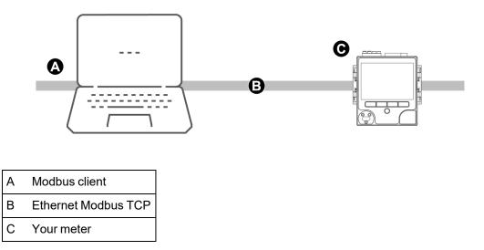
Your meter does not require any Modbus-specific configuration to act as a Modbus server device over Ethernet.
