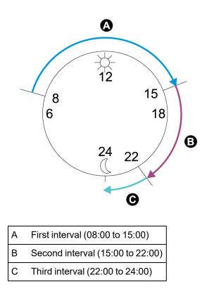
The first incremental energy interval is from 8AM (start time) to 3PM, and is 7 hours long. The second incremental energy interval is from 3PM to 10PM, and is also 7 hours long. The third interval is from 10PM to 12AM, and is only 2 hours long because 12AM is the specified end time. These intervals repeat every 24 hours until the configuration is changed or incremental energy feature is disabled.
